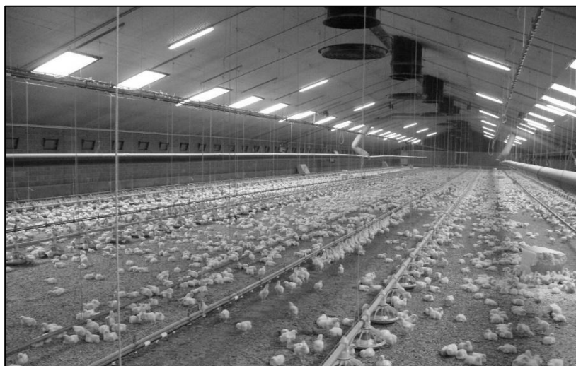
Figure 7. A 1515m 2 (approx. 18 x 85m) commercial broiler barn in the Netherlands equipped with two rows of 21 windows (total 42 windows) in the roof to allow natural light to enter. Each roof window measured 1.25m 2 , providing a total window area equalling 3% of the total floor space. Artificial lights on the roof are available to supplement daytime natural lighting as needed (Source: de Jong & Gunnink, 2019).
